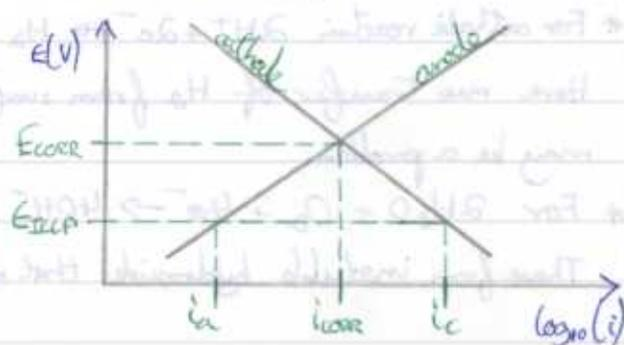
\* Can see that imposing a potential can make a metal either thermodynamically immune or reduce its corrosion rate by a great deal.
