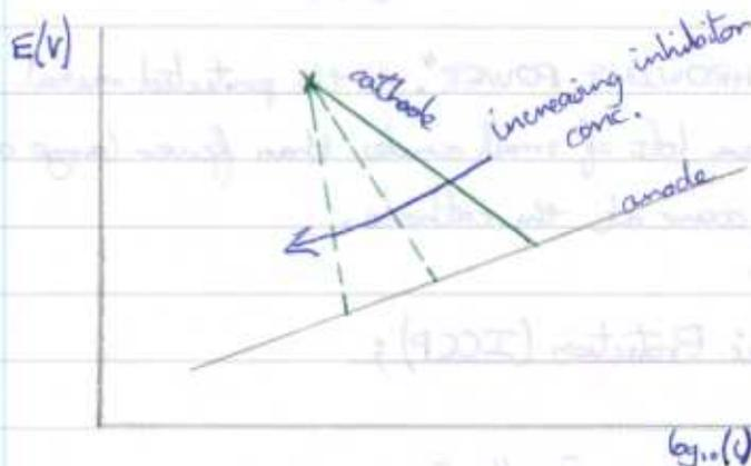
\* For cathodic reaction  $2H^+ + 2e^- \rightarrow H_2$ , inhibitors are As, Bismuth, Antimony ions. Here mass transfer of  $H_2$  from surface is reduced, so hydrogen embrittlement may be a problem.
